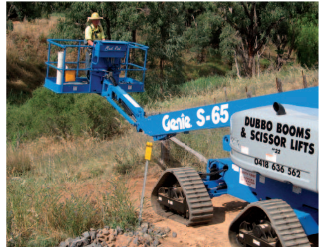
Dubbo Booms and Scissors Lifts (Mud Rat) S TM -85 telescopic boom with aftermarket Loegering quad-track system.
