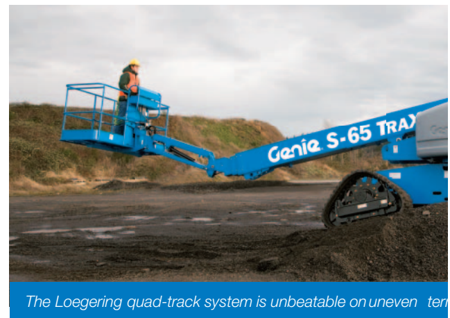
Dubbo Booms and Scissors Lifts (Mud Rat) S TM -85 telescopic boom with aftermarket Loegering quad-track system.
