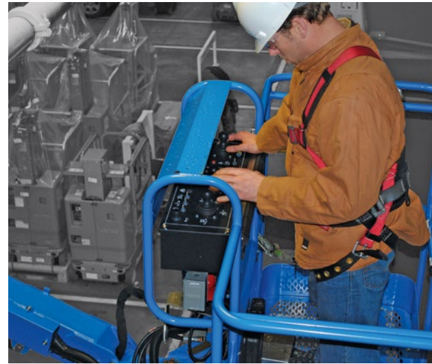
The OPA consists of a horizontally oriented sensing bar and reset button mounted adjacent to the platform control panel, plus a flashing strobe and horn mounted behind the platform controller.
