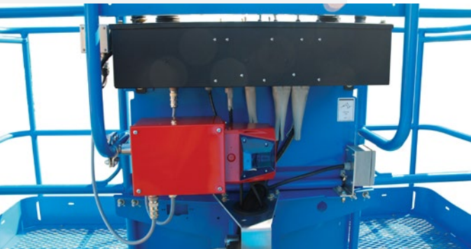
The Genie OPA is designed to be moved from machine to machine, rather than remain installed on a single machine.
