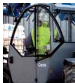
Door with 2 sections: steel on bottom, glass on top. Both sections open separately
