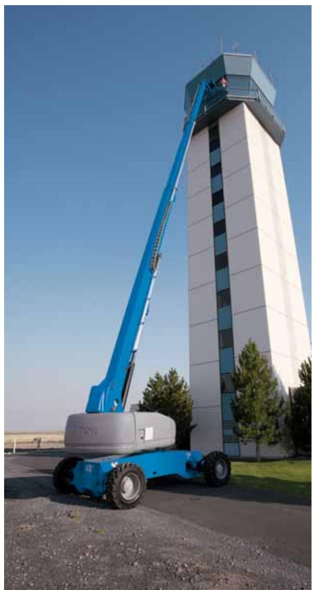
**The horizontal outreach of the Genie® Super Boom™ line is among the industry's best at 22.86 to 24.38 m (75 to 80 ft), depending on the model.**
