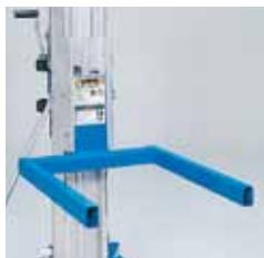
**STANDARD FORKS** accommodate a variety of general loads. Get an additional 51 cm (20 in) of lift by turning over and re-pinning the forks.
